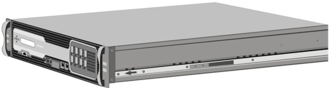
Figure 1. Attaching inner rails
